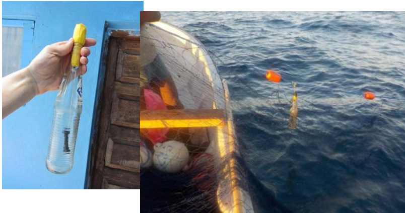
Fig. 2a and b. Glass bottle with pendulum metal bolt produce a sound similar to electronic pingers designed to reduce dolphin bycatch in gillnets.
