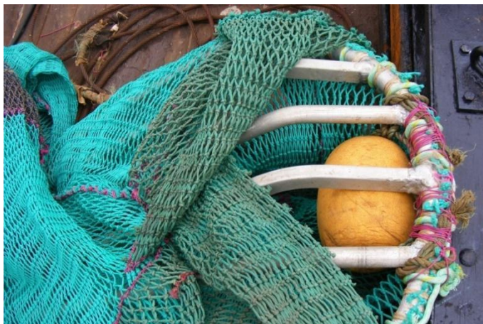
Figure 2: Double flaps (the dark green mesh which is folded back) are used to cover the escape opening; a single large float is used on this TED; there is a mixture of round and square bars in this TED
