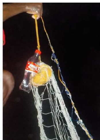
Figure 3 - Plastic bottle reflector attached to the sinkline, the device reflects echolocation clicks allowing detection of the nets by marine mammals.
