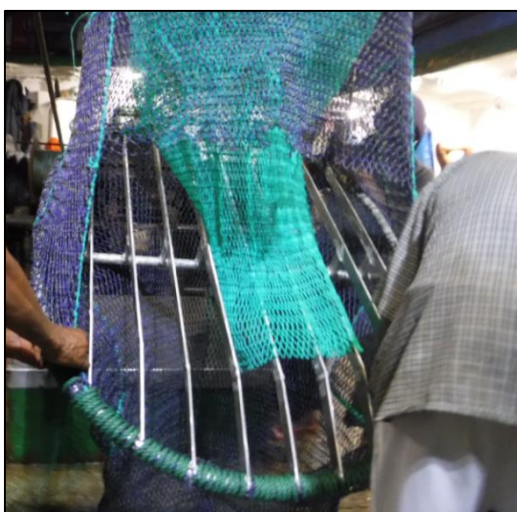
Figure 1: A flat bar super shooter TED grid being mounted into a TED extension
