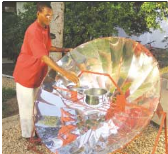
Solar cooker in use for boiling water.
